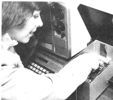
2. Here Jeri is setting the dip switches in The Solution. The hinged top makes the job easy. The switches can be set for three different things. Up to four boards can be installed inside the case.
